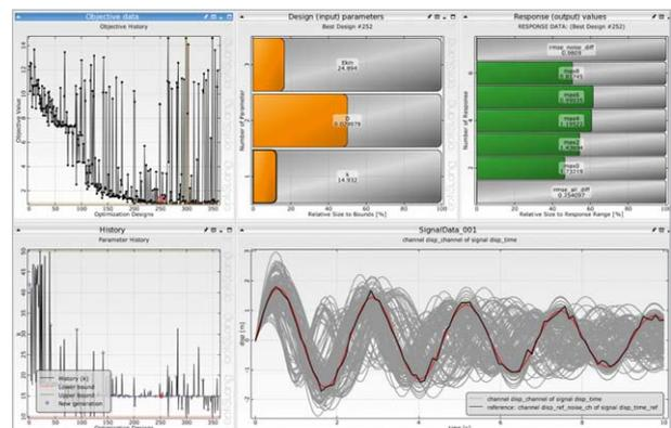
Figure 3: optiSLang signal post processing during the calibration process of a damped oscillator using evolutionary algorithms
