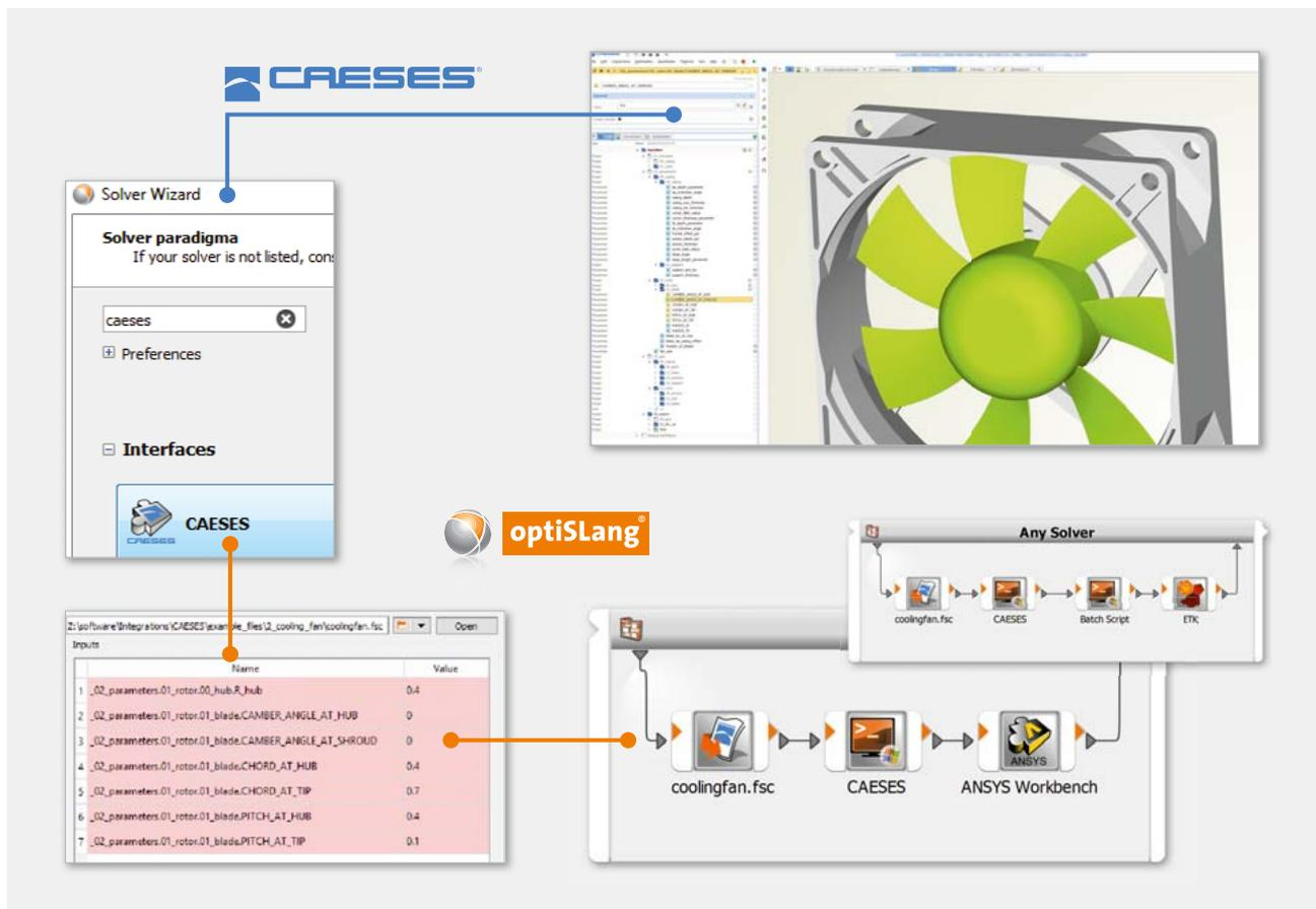
Setup of an automated simulation and optimization workflow using optiSLang, CAESES, ANSYS Workbench or other solvers
