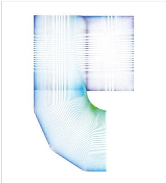
Fig. 1: Velocity profile of the initial diffuser
