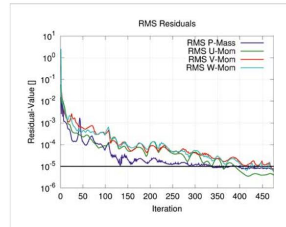
Fig. 4: RMS residuals of the CFD simulation.
