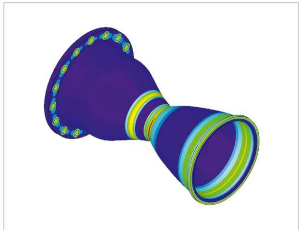
Fig.3: Accumulated plastic strain in the nozzle
