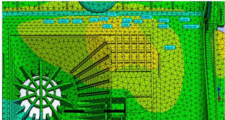
Deformation after non-linear analysis on the internal side of the compartment after 120s. Deformation is strongly reduced. Especially in the critical area values are decreased between 1.3 to 1.5 mm! This corresponds to a decline of 17-27% compared to the starting point!
