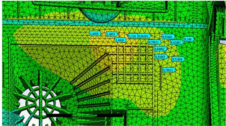
Parametric Design Optimization: The additional braces reinforce decisively the component in the relevant area. The area above the motor protection filter shows only small deformations below 1.5 mm, which corresponds to a reduction of 15-25% of the internal wall.
