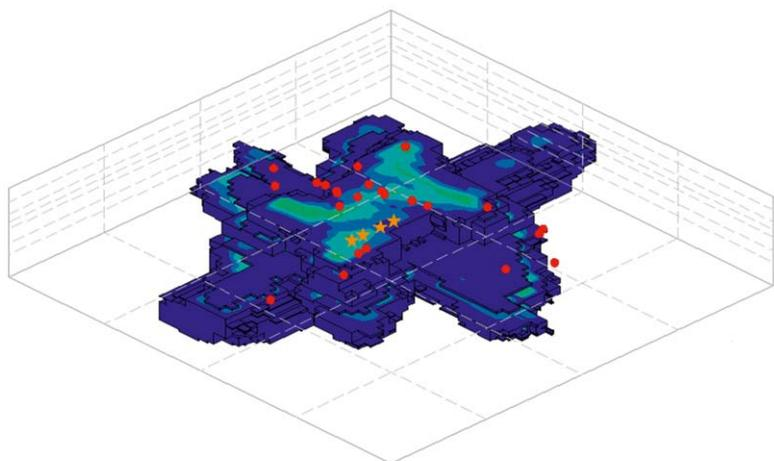
Stimulated rock body after 193 minutes compressive stress (blue=simulated/red=measured)
