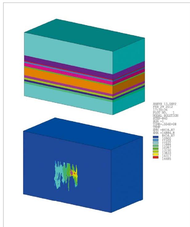
3D coupled thermal-hydraulic-mechanical FEM simulation of hydraulic fracturing
