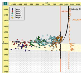
Comparison of simulation with measurements (Microseismic)
