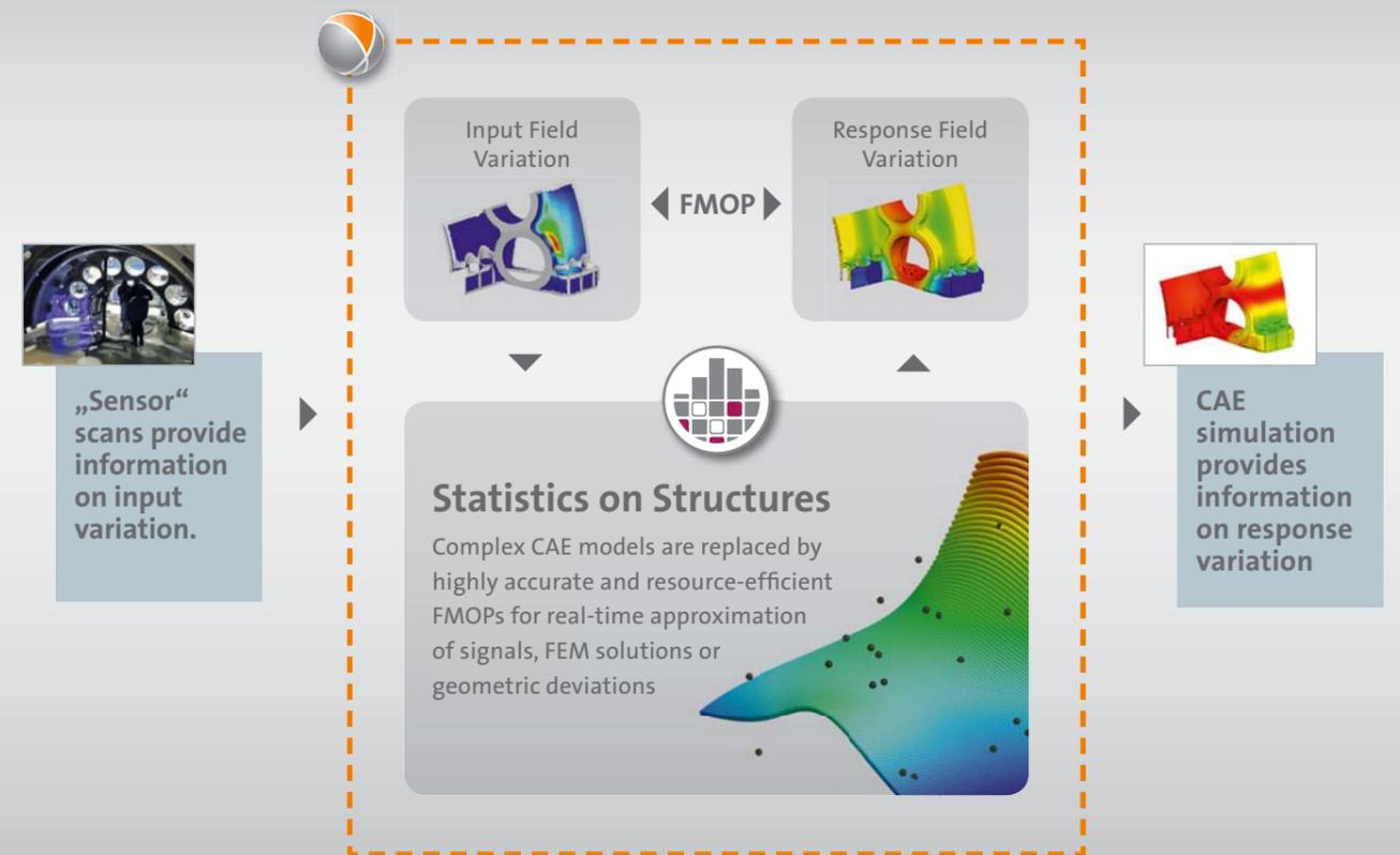
Workflow for the generation of a Field Metamodel of Optimal Prognosis (FMOP) connecting input and response field variation to be integrated in digital twins.
