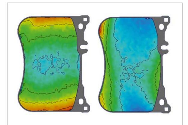
Picture of scatter shape parametric model of measured brake pad surfaces
