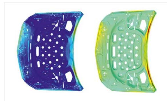
Standard deviation of response thickness variation after forming simulation (left) and the first scatter mode already representing 84% of the total variation (right)
