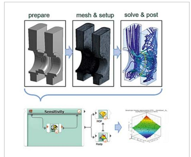
Fig. 6: Integration of ANSYS-Workbench (CFX) in optiSLang for MOP creation for the coupled system
