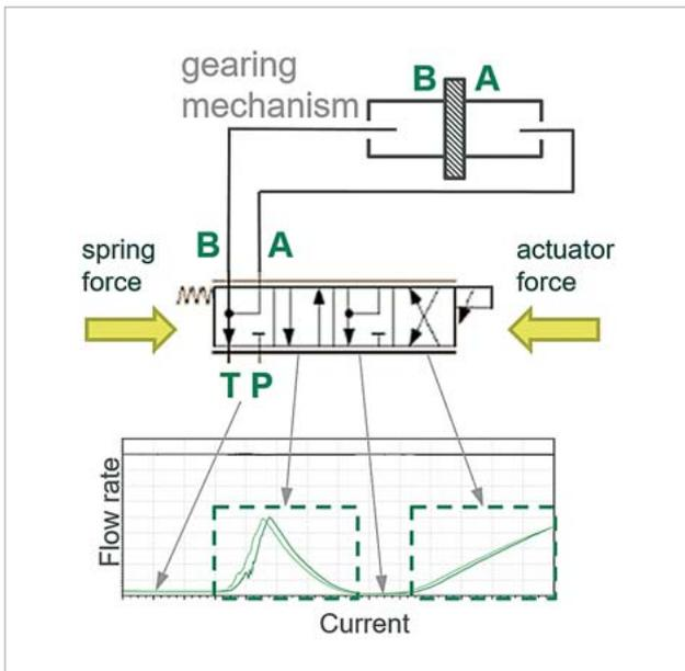
Fig. 1: Switching symbol and explanation of function including volumetric flow / flow-characteristic curve (Q-I)
