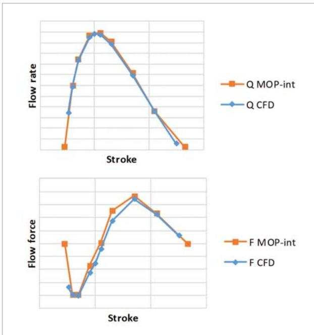
Fig. 10: Volume flow and flow force over the stroke for MOP interpolation and re-evaluated CFD simulation
