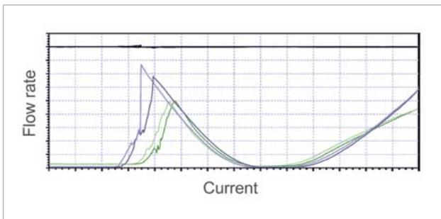
Fig. 11: Measurement results (Q-I characteristic) of the first prototypes (purple) compared to the reference (green)
