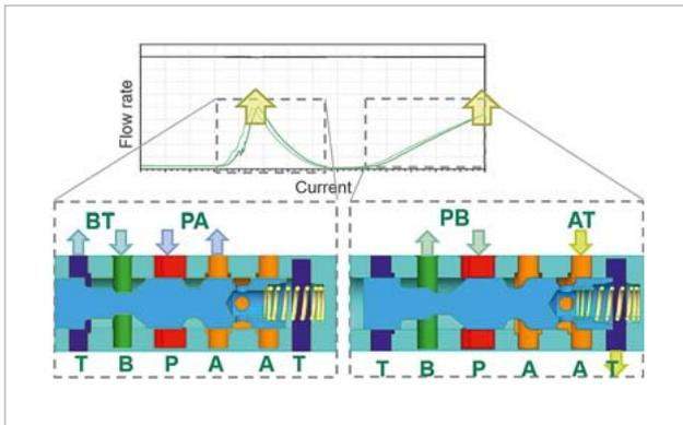
Fig. 2: Q-I characteristic curve with optimization target (yellow arrows) and valve geometry for the PA(BT) and PB(AT) switching positions
