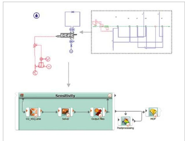
Fig. 3: System simulation model (AMESim, above) and integration into a sensitivity analysis in optiSLang (below)
