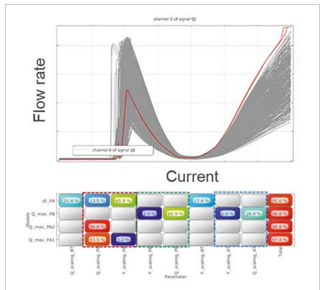
Fig. 4: Q-I characteristic curve variation (top) and COP matrix (bottom) for potential analysis
