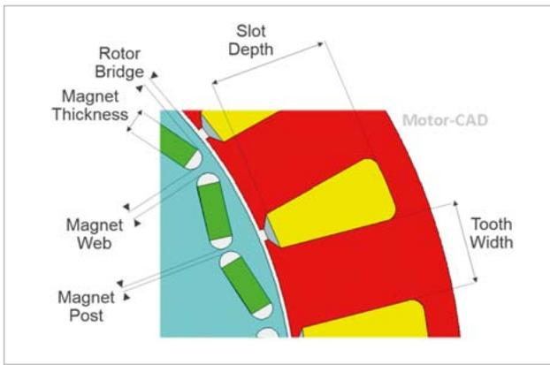
Fig. 1: Motor cross section geometry: Slot Depth Ratio = Slot Depth / (Slot Depth + Stator Back Iron Thickness) | Slot Width Ratio = Avg. Slot Width / (Avg. Slot Width + Stator Tooth Thickness) | Split Ratio = Stator Inner Diameter / Stator Outer Diameter
