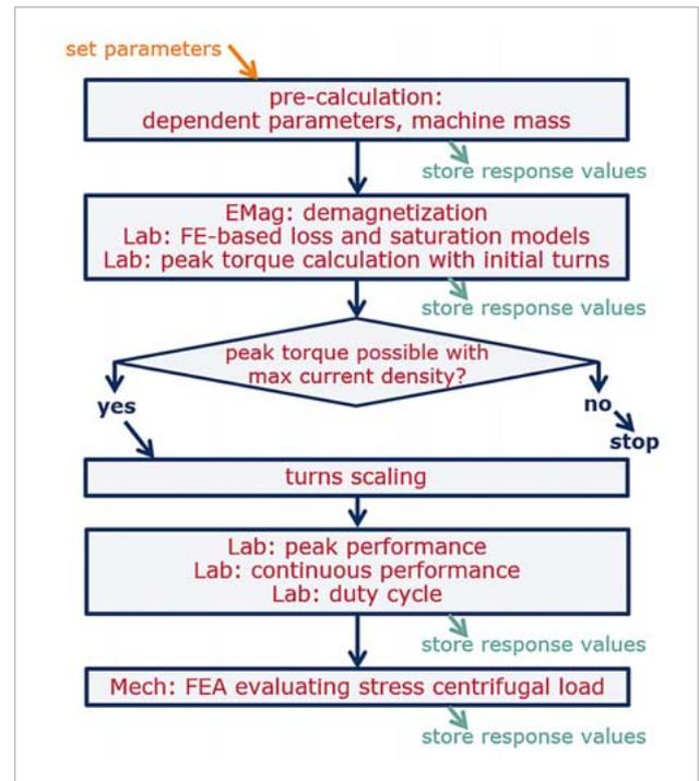
Fig. 2: Schematic of scripted Motor-CAD evaluation of one single design
