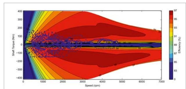
Fig. 4: Efficiency map with overlaid WLTP-3 duty cycle
