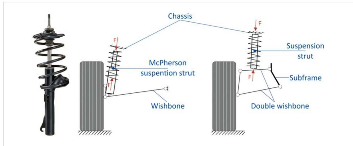
Fig. 1: Spring arrangement around the damper
