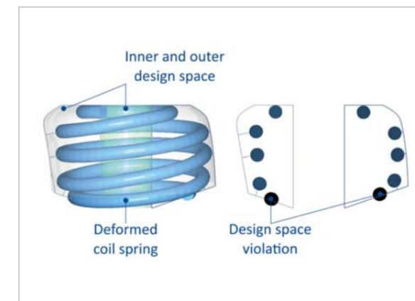
Fig. 5: Inner and outer design space limits (left) and section through design limits and coil spring (right)
