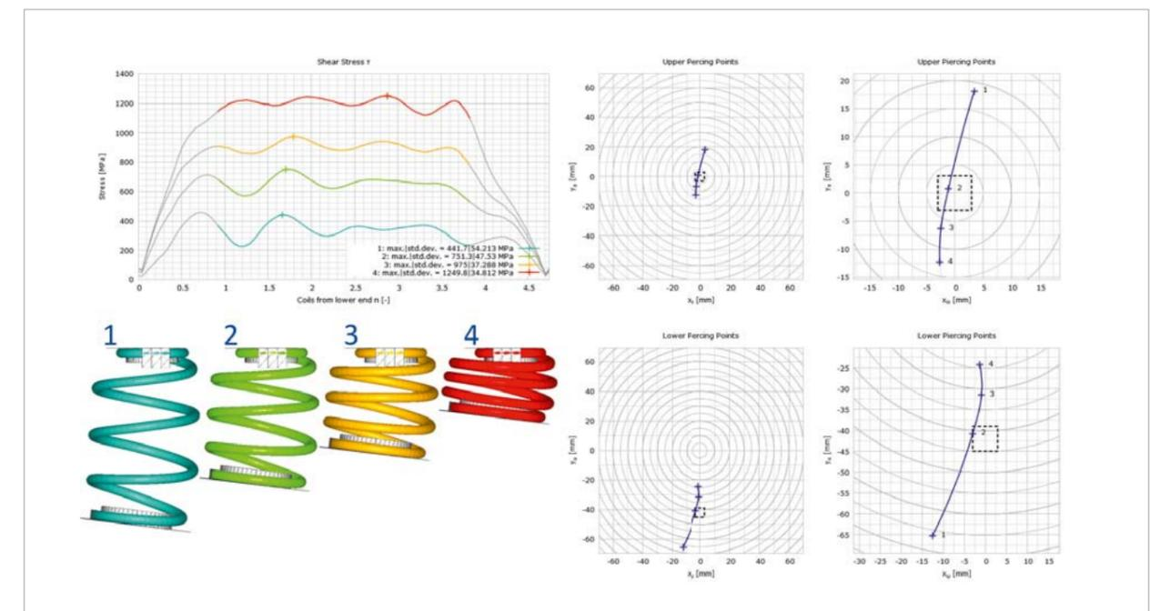
Fig. 7: Shear stress curve (left) and piercing points (right) in different compression states
