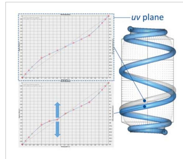
Fig. 4: Generation and variation of the coiling in the uv-plane
