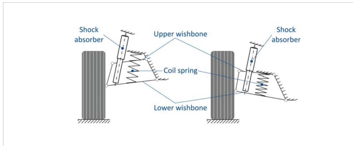
Fig. 2: Spring arrangement on a wishbone: decompressed (left) and compressed (right)
