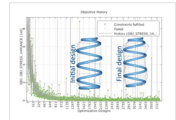
Fig. 6: Initial cylindrical coil spring design and final geometry
