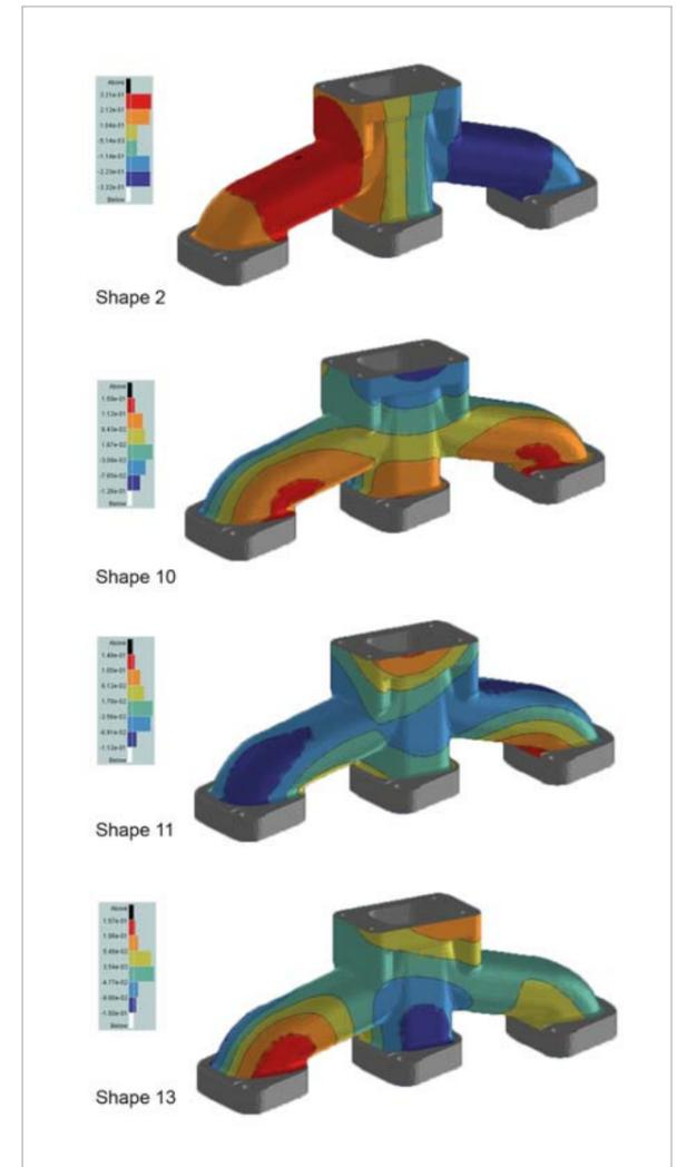
Fig. 6: Metamodel of Optimal Prognosis for minimum life location
