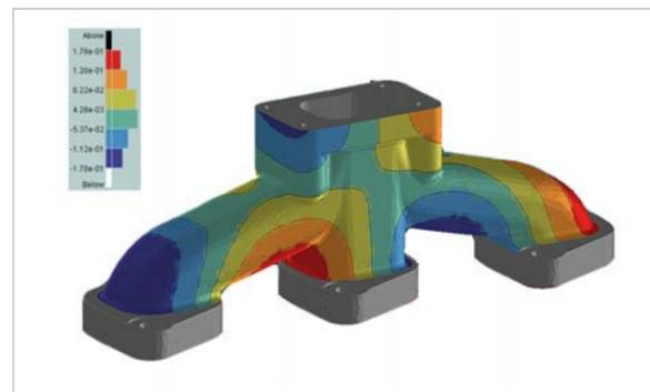
Fig. 4: Eigen shape contour showing normal movement of node
