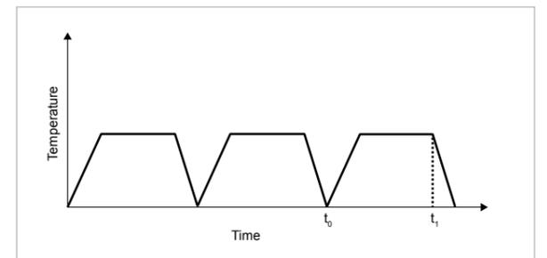
Fig. 1: Time points selected to find the difference in stress tensors
