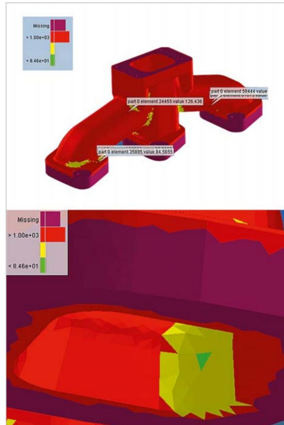
Fig. 5: 95% quantile plot for fatigue life
