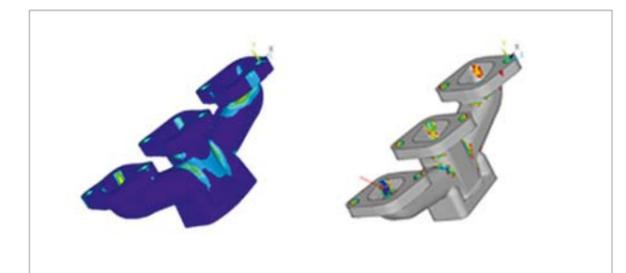
Figure 3: Plastic strain (left) and life plot (right)
