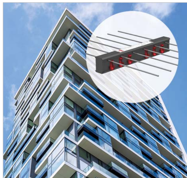
Fig. 3: HALFEN HIT ISO-element HIT-HP/SP MVX for the thermally insulated connection of balconies and projecting cladding parts
