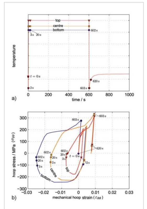
Fig. 3: Stress strain hysteresis in the hot wall ligament during the first load cycle: a) Transient temperatures; b) Stress-strain response in different locations through the liner ligament [5]
