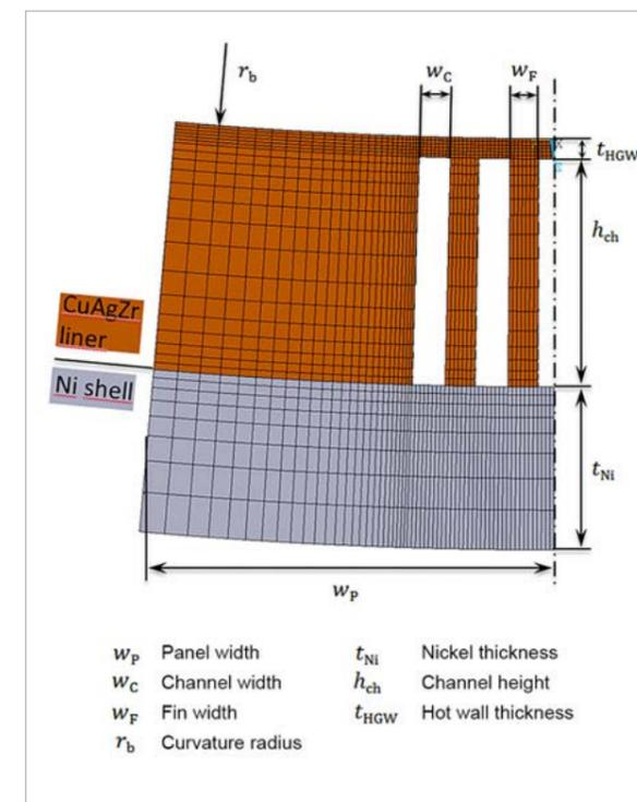
Fig. 6: Modified geometry parameters defining the panel design
