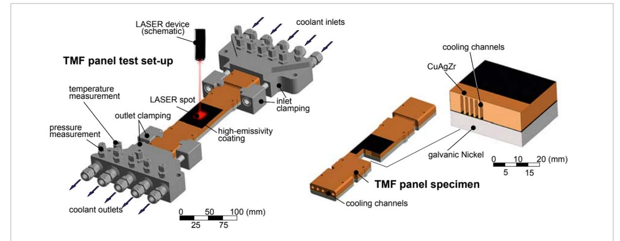
Fig. 2: TMF panel design and test concept [5]
