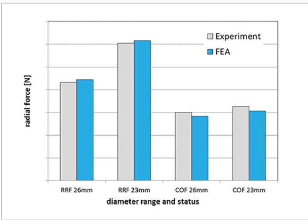
Fig. 3a: Comparison of experimental vs numerical radial force results for an exemplified stent design in a 23mm and 26mm vessel model
