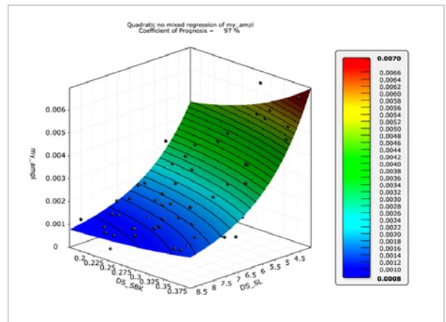
Fig. 4b: Strain amplitude as function of strut length (SL) and strut thickness (SBK)
