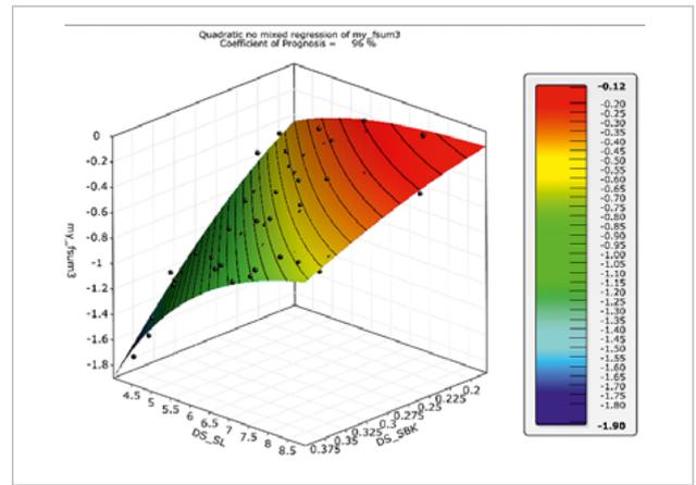
Fig. 4a: Radial force as function of strut length (SL) and strut thickness (SBK)
