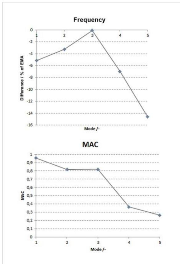
Fig. 4: Comparison of the Experimental Modal Analysis (EMA) with the simulation of the bar
