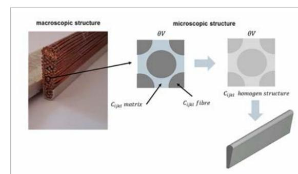
Fig. 2: Homogenization
