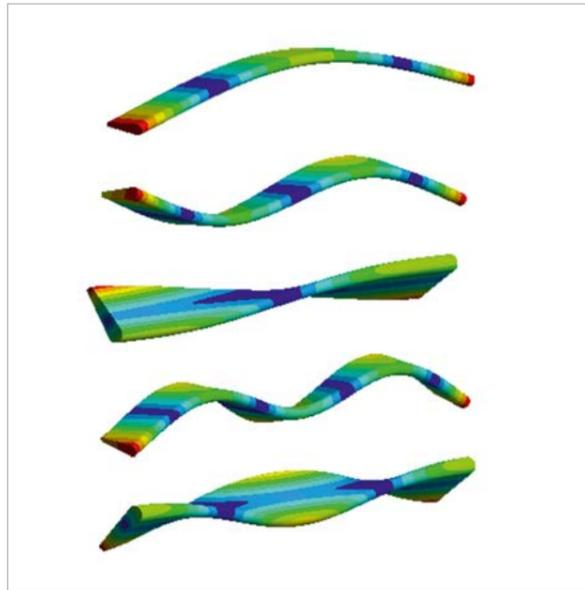
Fig. 3: Mode shapes of the slot bar | top down - 1st bending, 2nd bending, 1st torsion, 3rd bending, 2nd torsion
