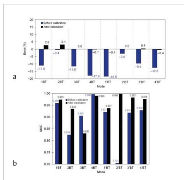
Fig. 9: Comparative analysis of the errors of experimental and numerical responses, before and after calibration: (a) vibration frequencies; (b) MAC
