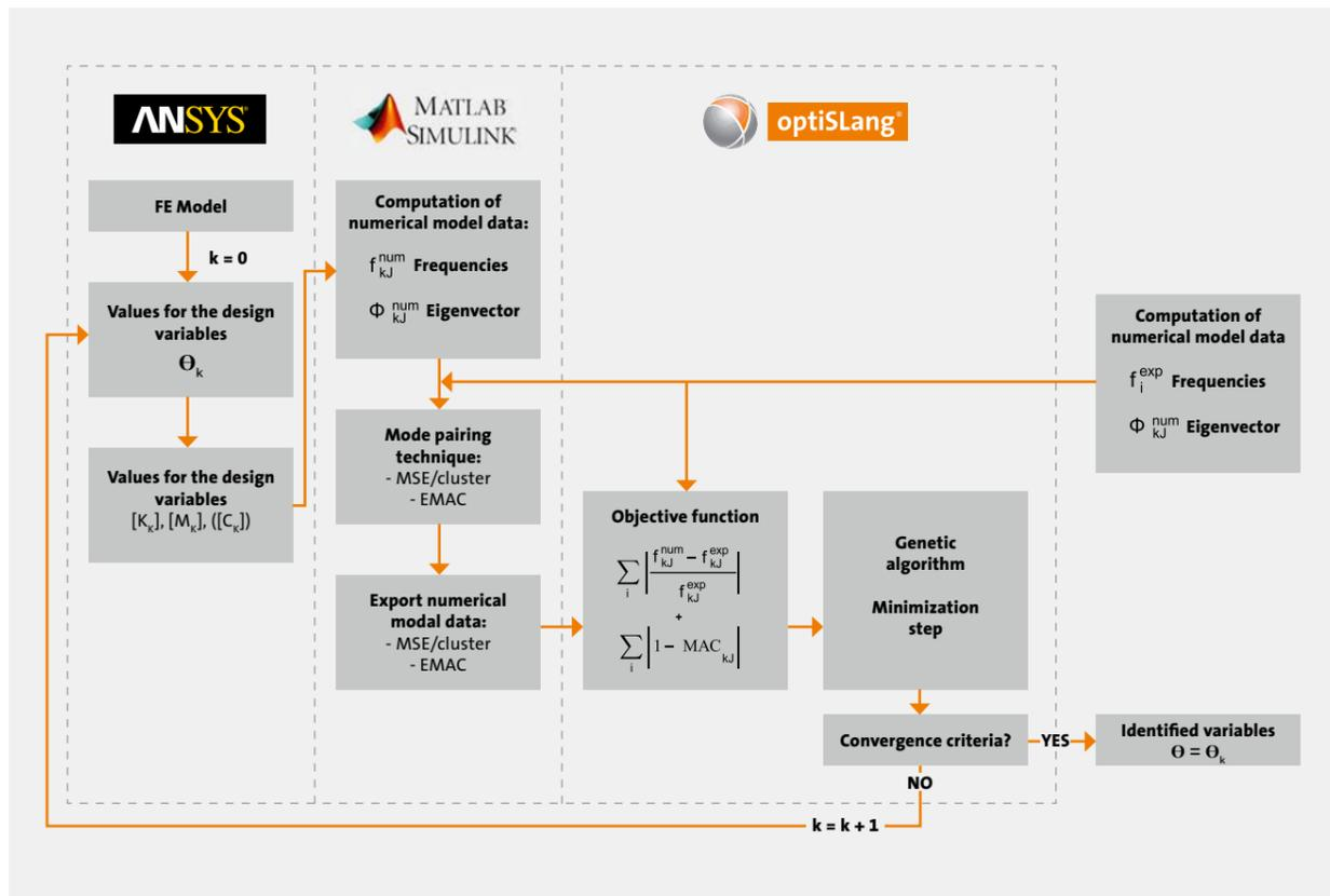
Fig. 6: Calibration methodology for the numerical model
