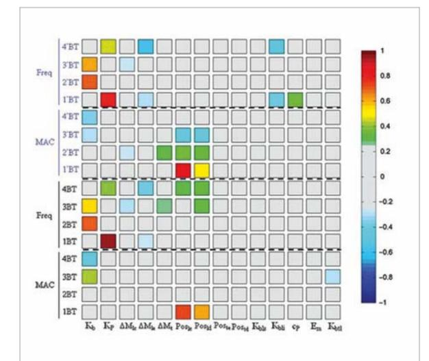
Fig. 7: Spearman's rank correlation coefficient between the parameters and responses of the numerical model of the bogie under test conditions
