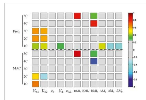
Fig. 11: Spearman's rank correlation coefficient between the parameters and responses of the carbody's numerical model
