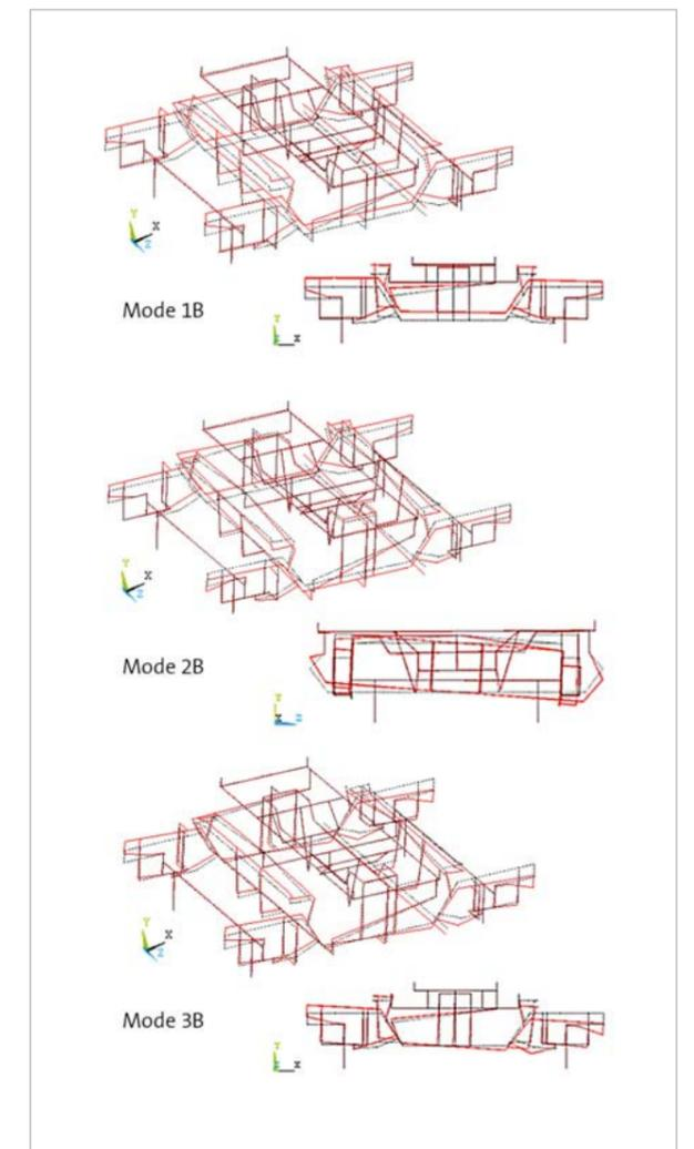
Fig. 5: Numerical modes of vibration of the bogies
