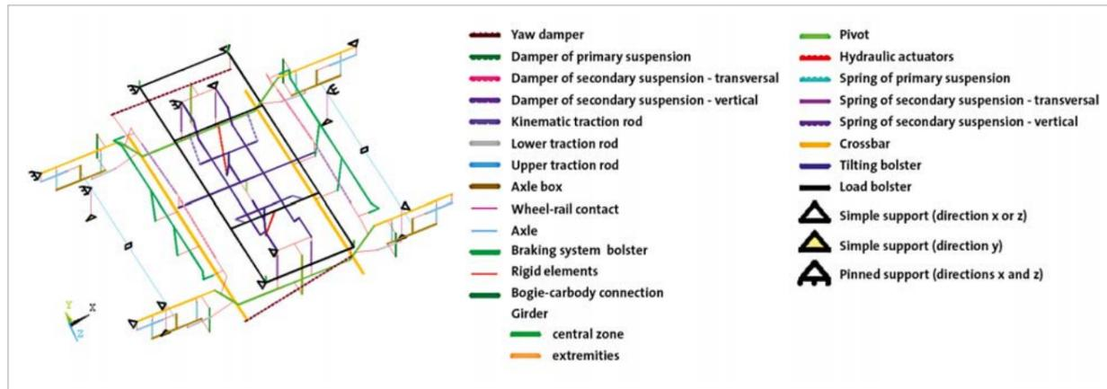
Fig. 3: Numerical model of the bogie
