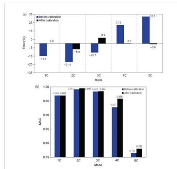
Fig. 13: Comparative analysis of the errors from the experimental and numerical responses, before and after calibration in terms of: (a) vibration frequencies; (b) MAC
