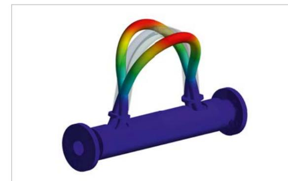
Fig. 2: Fundamental oscillation of the measuring tubes at about 100 Hz and a few micrometers of deflection (shown in heightened form).
