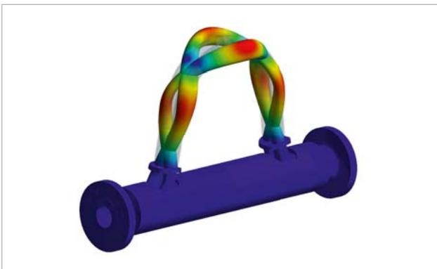
Fig. 4: Harmonic component at about 1000 Hz (deflection shown in heightened form)
