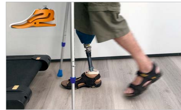
Fig. 1: Patient fitting and rehabilitation with a 3D-printed Mecuris prosthetic foot. The foot displayed is inserted into a cosmetic shell
