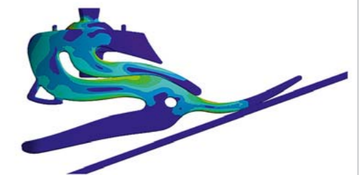
Fig. 2: ISO 10328 test stand and modeling of the two load cases with the subject prosthetic foot. All construction components are included in the FE-simulation (equivalent stress is shown)
