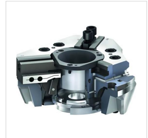
Fig. 6: The axially displaceable piston transmits the force to the base jaws and generates a radial jaw movement synchronous to the axis of rotation
