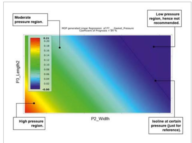
Fig. 13: Pressure distribution on bridge region
