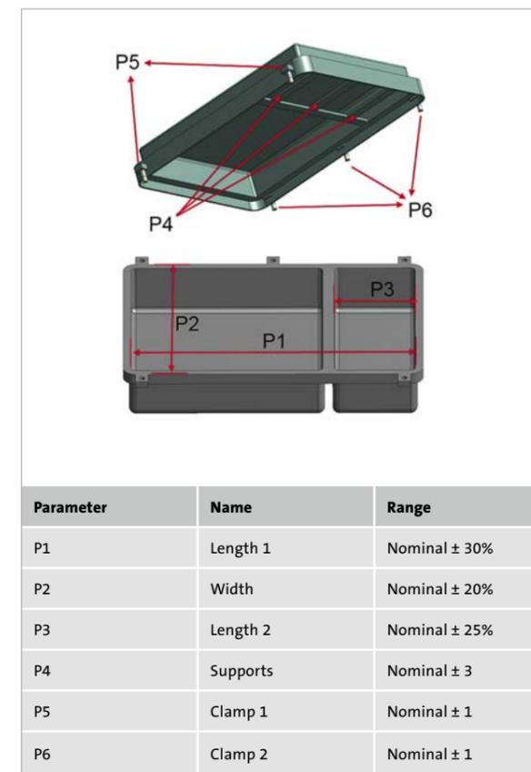
Fig. 9: Parameters and their range for seal profile optimization (reference model)
