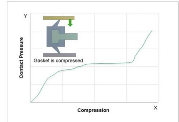
Fig. 10: Closure versus pressure curve (reference model)
