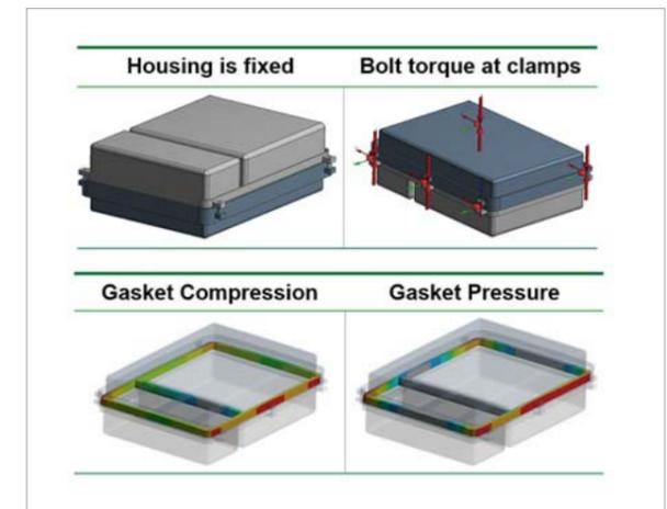
Fig. 11: Boundary conditions, gasket compression and gasket pressure
