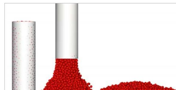
Fig. 1: Illustration of the transient simulation to determine the angle-of-repose and the draw-down angle of a bulk material
