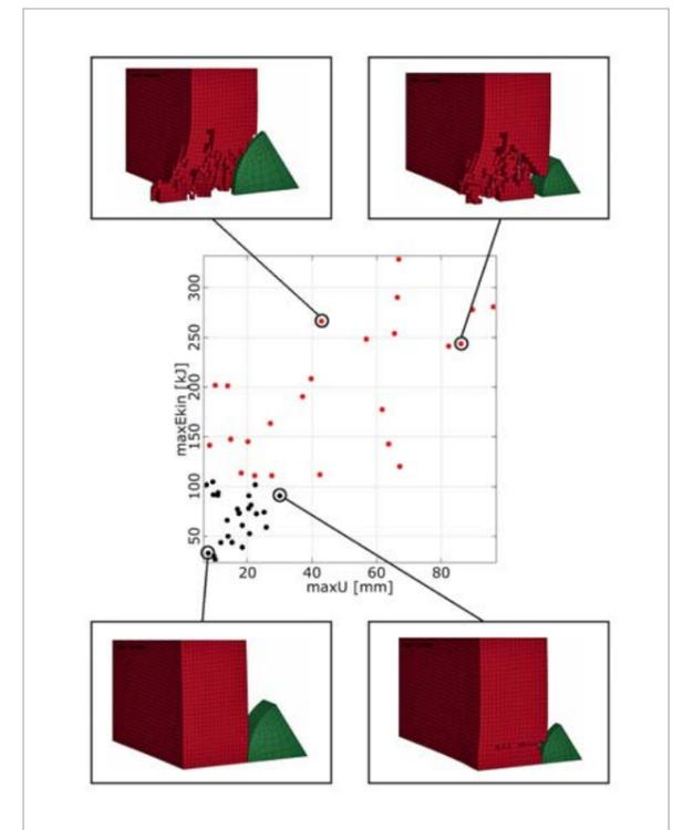
Fig. 6: Pairwise dependence of the kinetic energy regarding the penetration depth
