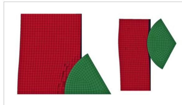
Fig. 4 Sample plots for the state of final deformation regarding an impact area located in the middle and at the upper edge
