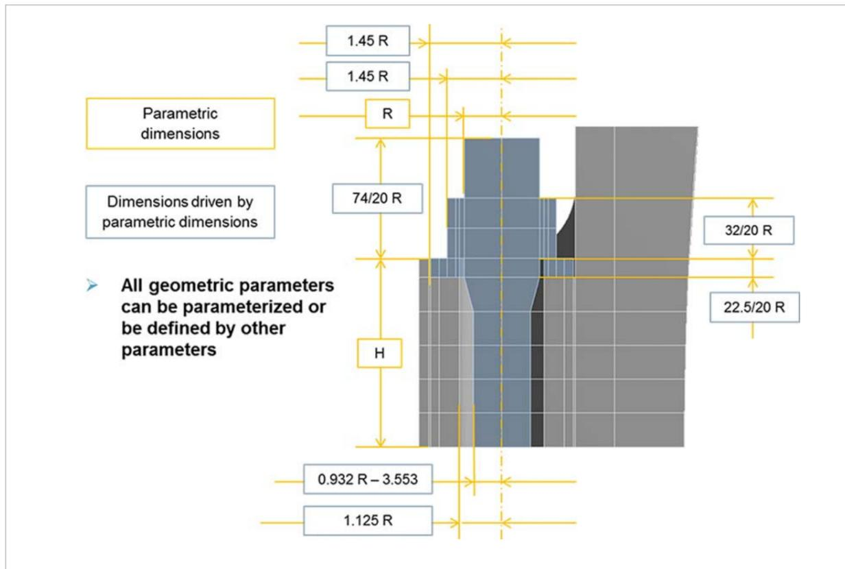
Fig. 3: Parameterization of the geometry
