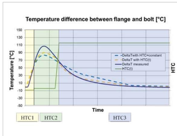
Fig. 11: Temperature difference between flange and bolt
