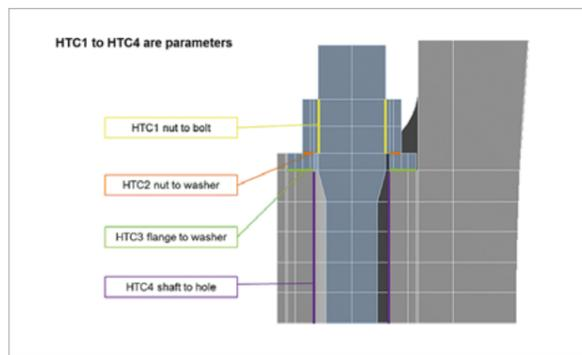
Fig. 4: Definition of heat transfer coefficients
