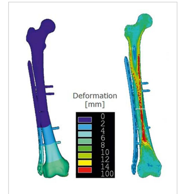
Fig 11: Optimal design after optimization under pre-defined constraints. The optimal design consisted of four screws in total, two screws on the distal segment and two screws on the proximal segment. The bridging length measured 100 mm
