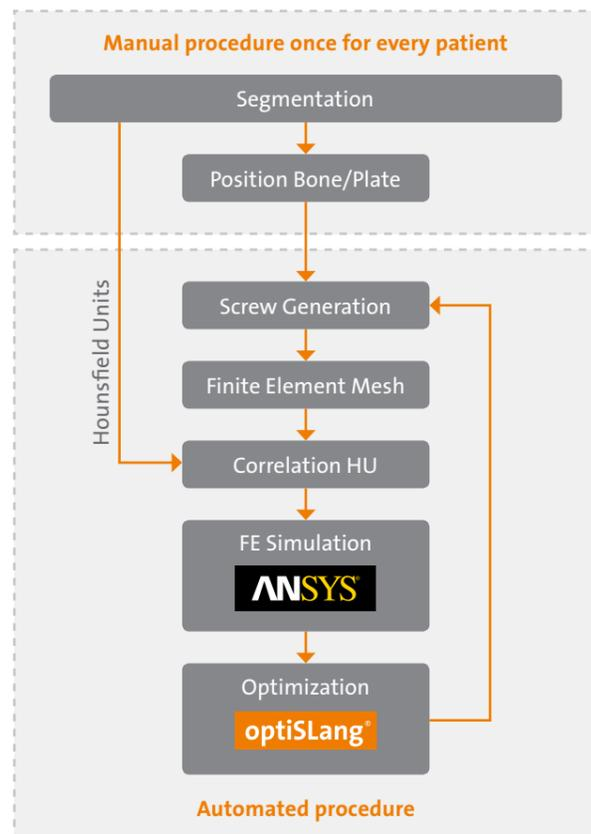
Fig. 2: Procedure for the optimization of fracture treatment
