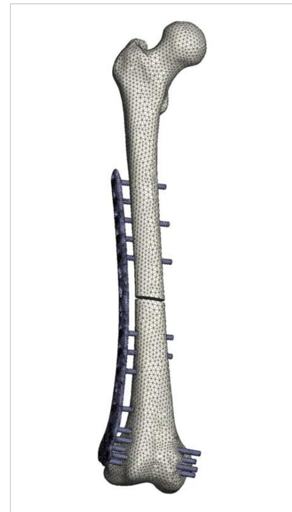
Fig. 5: Meshed bone with plate and screws
