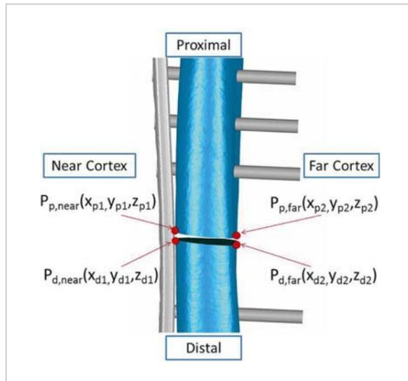
Fig. 7: Determination of interfragmentary movement using the relative displacement of two points on the far cortex and on the near cortex of the bone. ( $P_{p,xxx}$  = Displacement of node on proximal bone fragment,  $P_{d,xxx}$  = Displacement of node on distal bone fragment,  $d$  = Relative displacement between two points)
