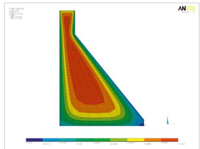
Fig. 1: Estimated temperature distribution after RCC placement
