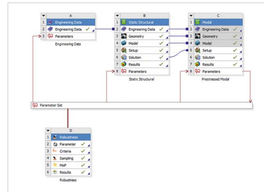
Figure 4: Brake squeal simulation process with ANSYS Workbench and optiSlang.
