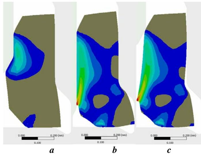
*Fig. 5: Typical results for the equivalent plastic strain in the Hyrel joint a) during the driving process b) with the glass mounted c) after having removed the glass. All plots use the same scale.*
