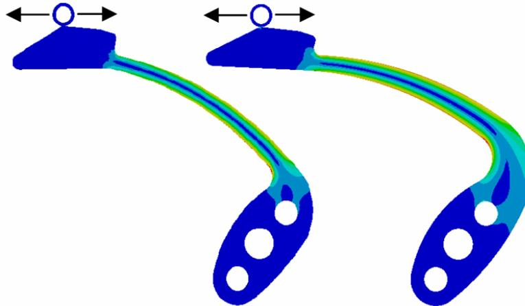
*Fig.2: Spring initial shape (left) and tuned shape (right). The pin of the pull-out piece is at the force inversion position where stresses reach their maximum. The positioning and angle of the two flat contact faces of the spring determine the pull and push forces.*
