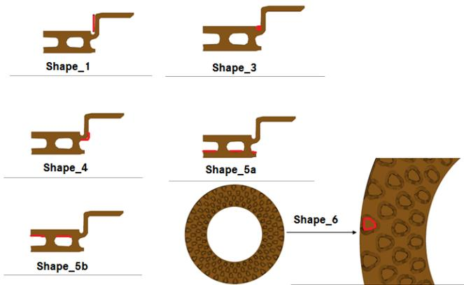
Figure 4. Parametrization of brake disc geometry using morphing functions (geometric variation windows marked in red)
