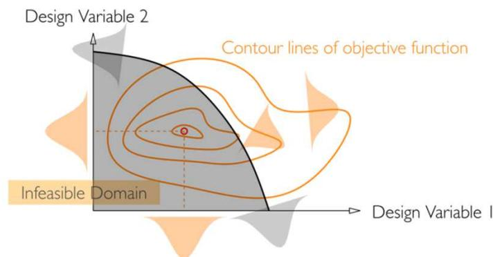
Figure 3: Robust Design Optimization: Optimization considering uncertain input parameters and responses as well as uncertain objective and constraint functions
