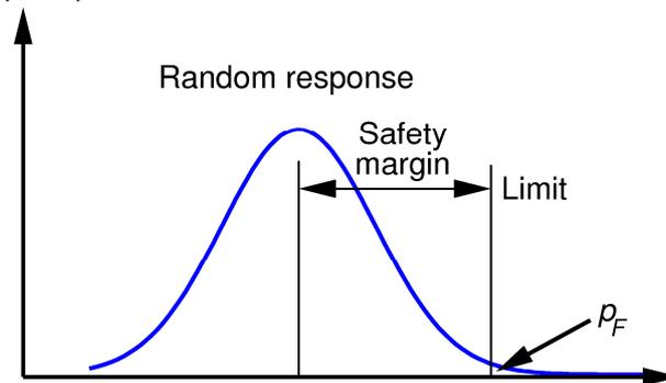
Figure 1: Scatter of a fluctuating response with safety margin (distance between mean and the failure limit) and the corresponding probability of failure  $p_F$
