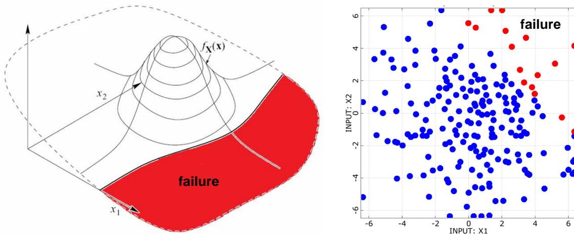
Figure 2: Reliability analysis as multi-dimensional integration of the probability density of the inputs uncertainties over the failure domain (left) and integration by Monte Carlo Simulation (right)
