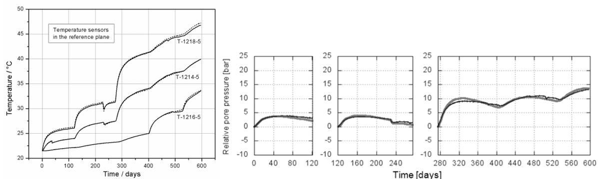
Figure 4: Comparison of calculated best design with measured signal: left) temperature evolutions for three selected sensors. right) relative pore pressures versus time at TED 1258
