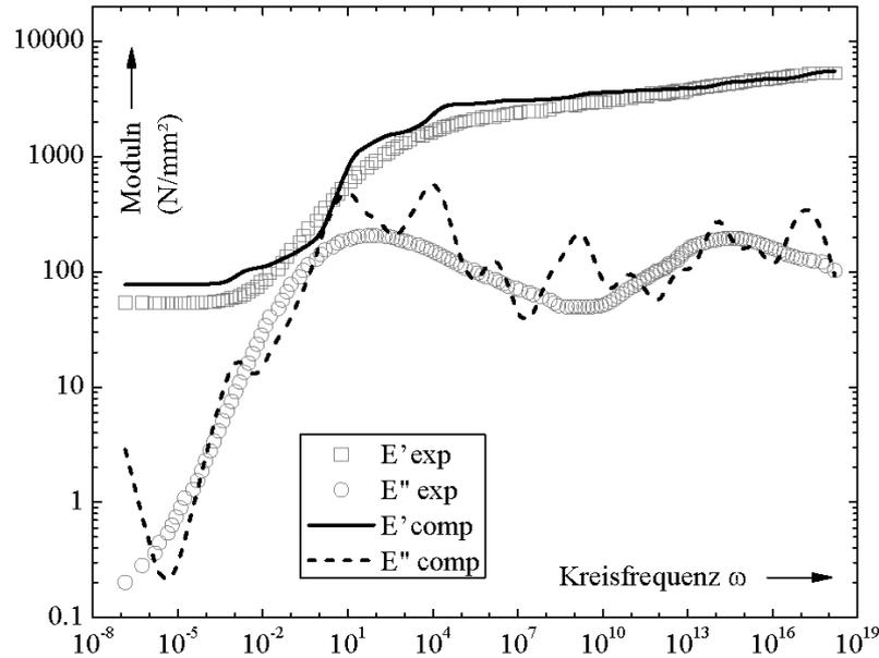
Fig. 7 Calibration of measurement and computation using an automated genetic optimization strategy
