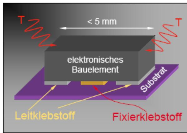
Fig. 6 Adhesive joints of electric components
