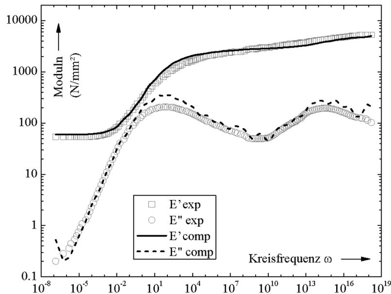
Fig. 8 Calibration between measurement and computation via automated genetic optimization strategy and subsequent gradient based mathematical
