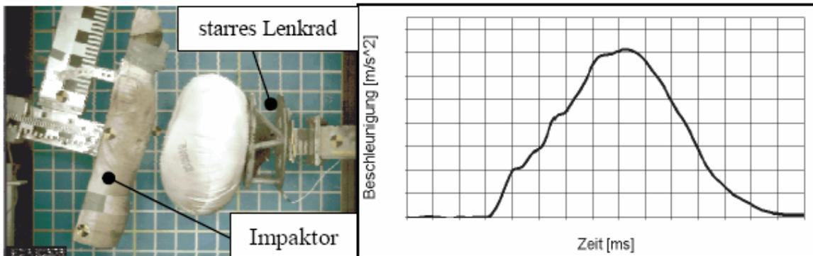
Abb. 9: Impactor test (left) und acceleration characteristics (right)
