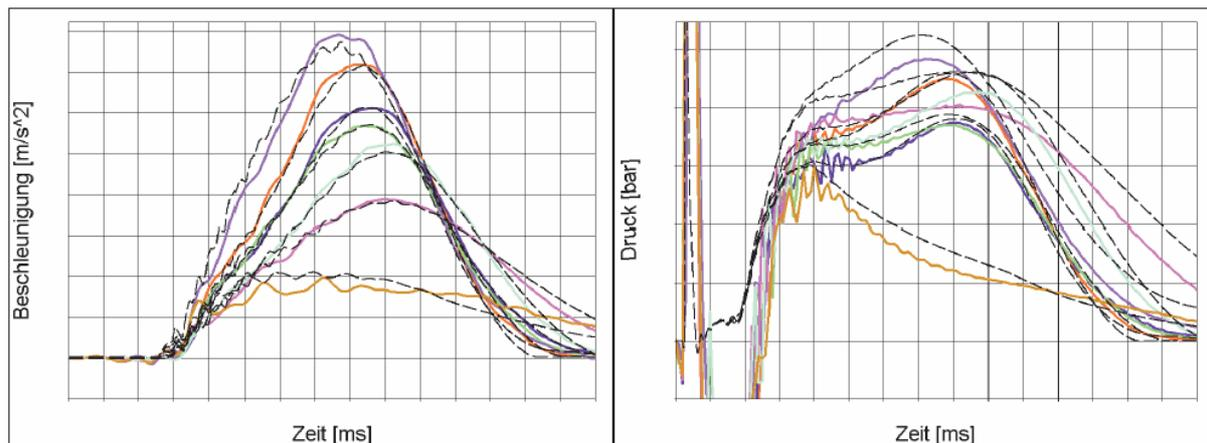
Fig. 11 Comparison of the acceleration and pressure runs from the experiment (coloured, drawn through) computation (black, dashed)
