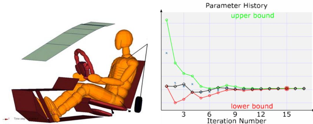
Fig. 1 Occupant restraint system and convergence of the adaptive response surface. After ten approximations, all parameters had converged.
