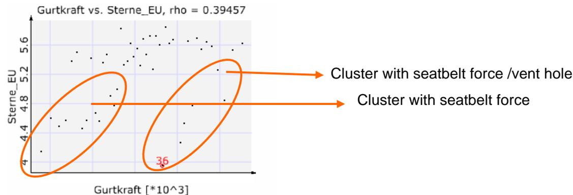
Fig. 2 Anthill plot seat belt force versus EURO NCAP evaluation. The two decreasing clusters illustrate two mechanisms of performance loss.
