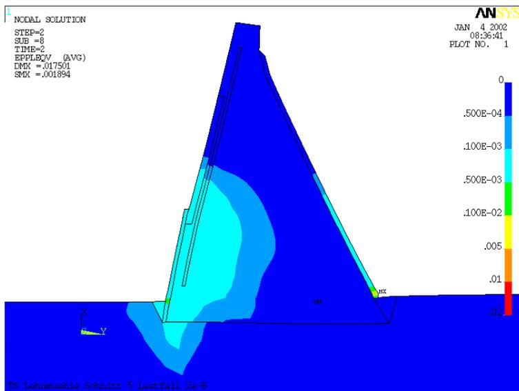
Fig. 13 Plastic strain
