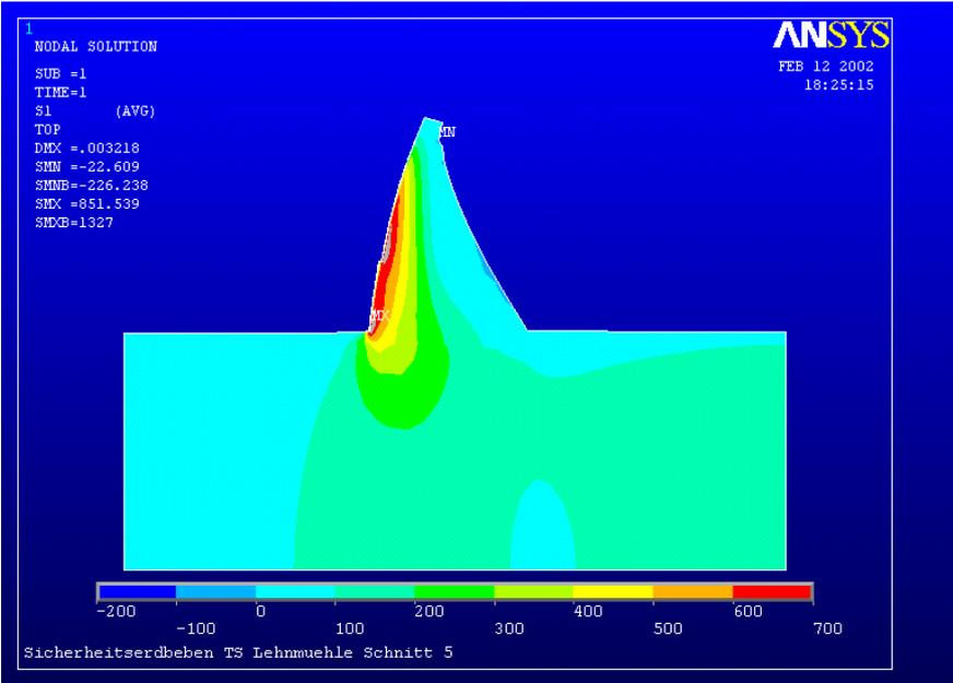
Fig. 8 Main tensile stresses [KN/m<sup>2</sup>] from the linear superposition of three modes
