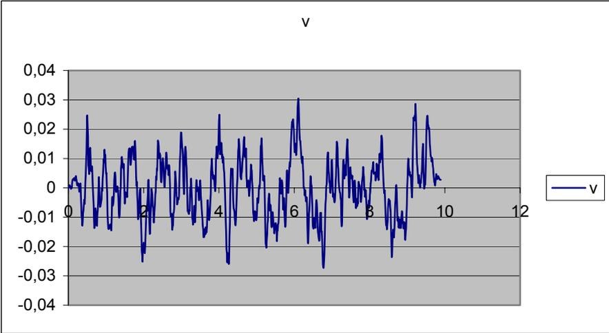
Fig. 9 Speed function of the strong quake phase in m/s
