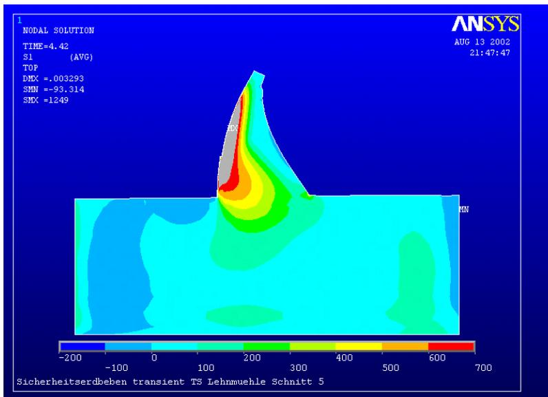
Fig. 11 Tension field of the maximal main tension load from the transient earthquake calculation
