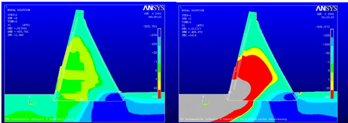
Fig. 15 Main tensile stresses [in KN/m<sup>2</sup>] for the elasto-plastic calculation (left) and the comparative elastic calculation (right)
