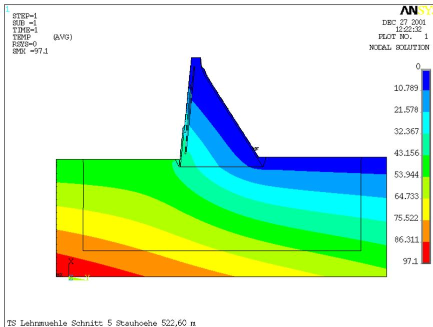
Fig. 3 Water pressure field [meter water column] operational water level with effective drainage
