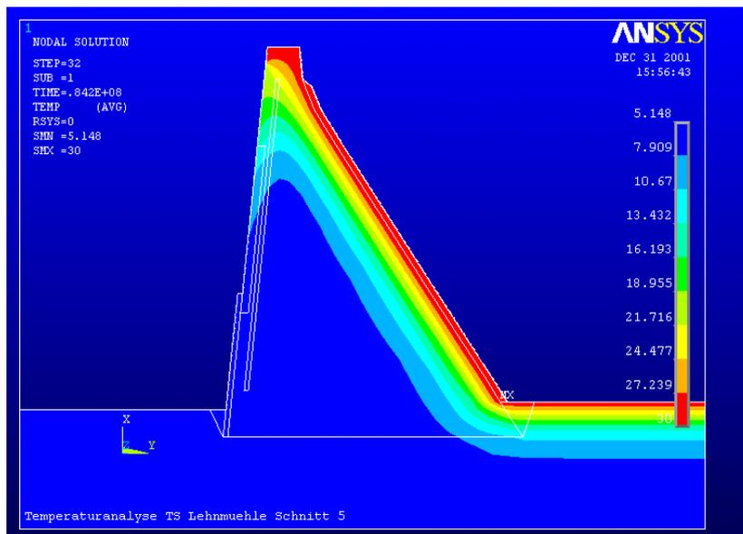
Fig. 6 Temperature field [in °C] with the greatest crown displacement (rare temperature occurrence in summer)
