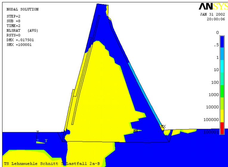
Fig. 14 Plastic activity (Yellow – tensile activity; Light blue –shear activity)
