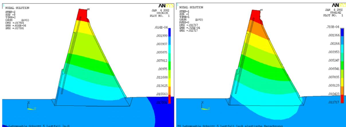
Fig. 12 Total displacement of the elasto-plastic calculations (left) and the elastic comparison calculations (right)
