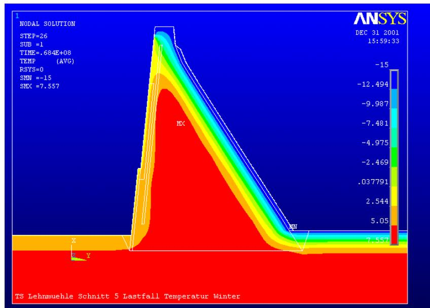
Fig. 5 Temperature field [in °C] with the greatest crown displacement (rare temperature occurrence in winter)
