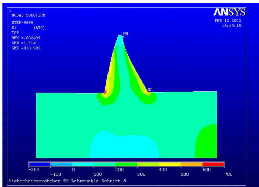
Fig. 7 Main tensile stresses [KN/m<sup>2</sup>] from the quadratic superposition of three modes
