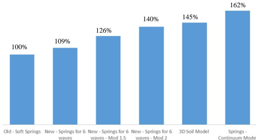
**Figure 5** Suction capacity obtained with the different soil/spring stiffness
