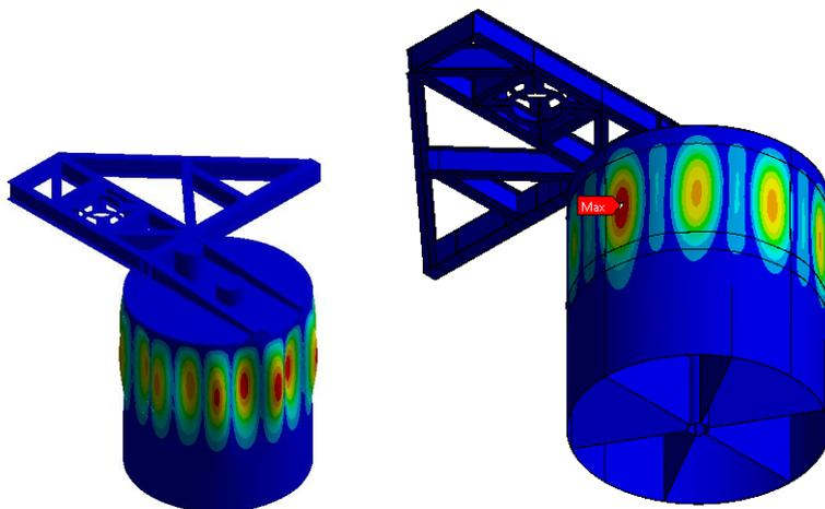
**Figure 2** Buckling mode (left) radial displacement at structural collapse (right)
