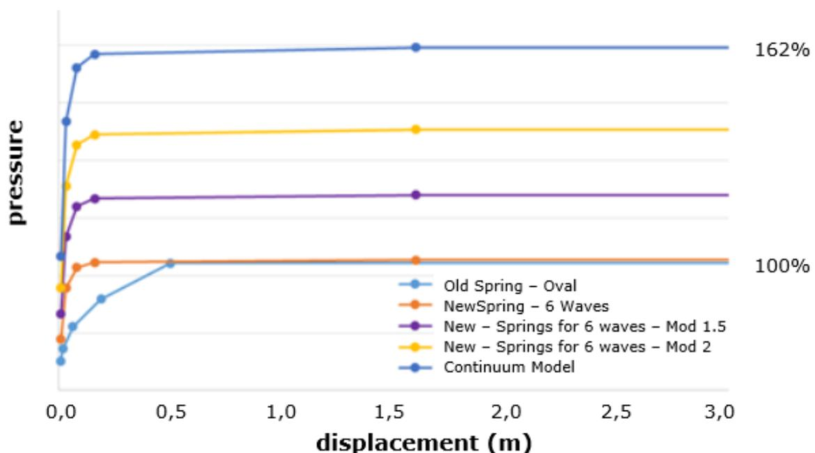
**Figure 4** Non-linear spring stiffness used in the results validation
