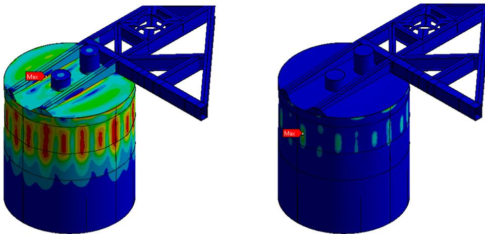
**Figure 3** von Mises Stresses (left) equivalent plastic strain at structural collapse (right)
