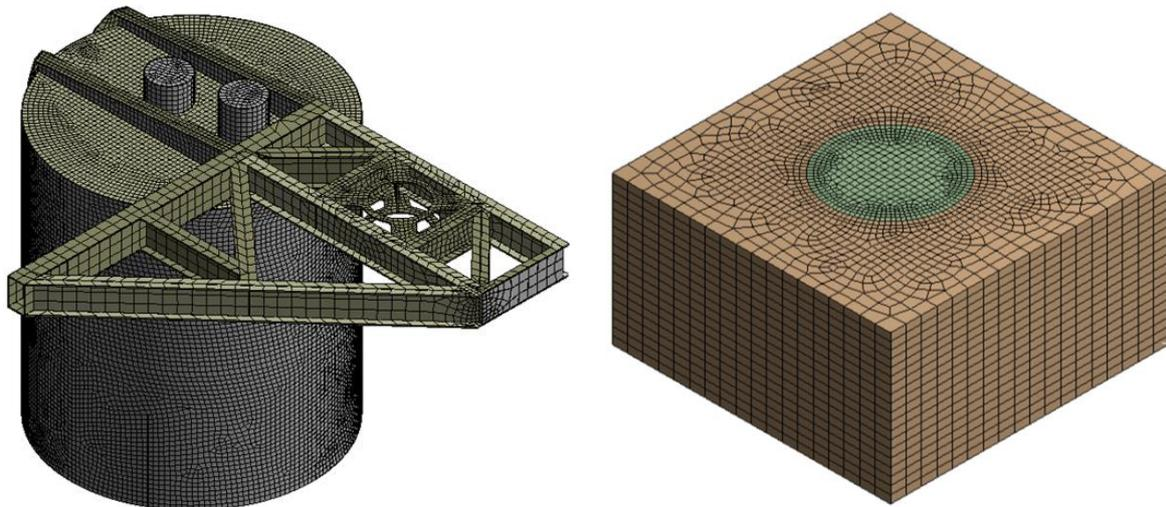
**Figure 1** Finite Element Mesh of suction pile (left) and soil (right)
