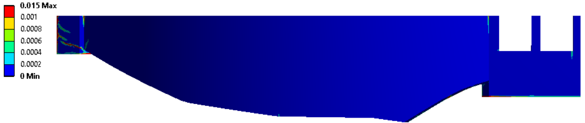
Figure 14: Upstream view of equivalent plastic strains at the end of the simulation (2 Years, Cold-Warm Year); Red areas are subjected to cracks ( \epsilon_p > 0.3\% plastic strain). Comparison between the linear and nonlinear results
