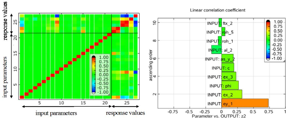
Figure 6: Left: linear correlation matrix, service load level; right: linear correlation coefficients, response  $z2$ – relative vertical displacement of the arch crown
