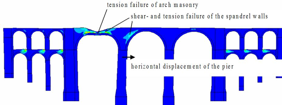
Figure 9: plastic strains and failure mechanisms
