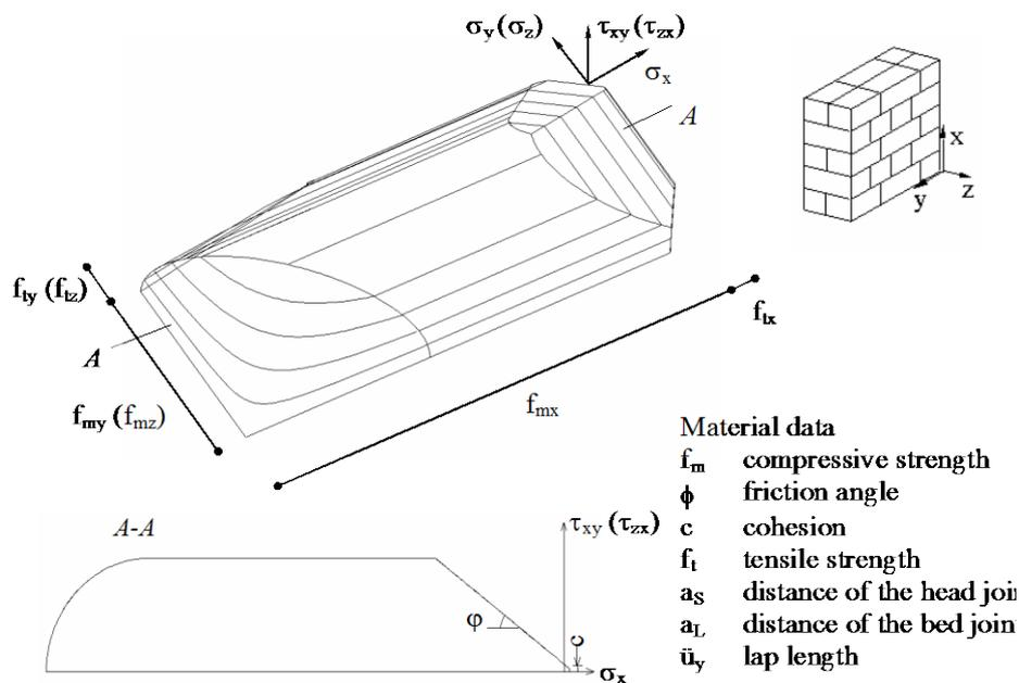
Figure 1: Yield criterion for regular masonry.
