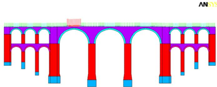
Figure 4: Relevant life load position
