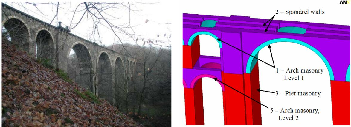
Figure 3: Masonry arch bridge (left), material areas (right)
