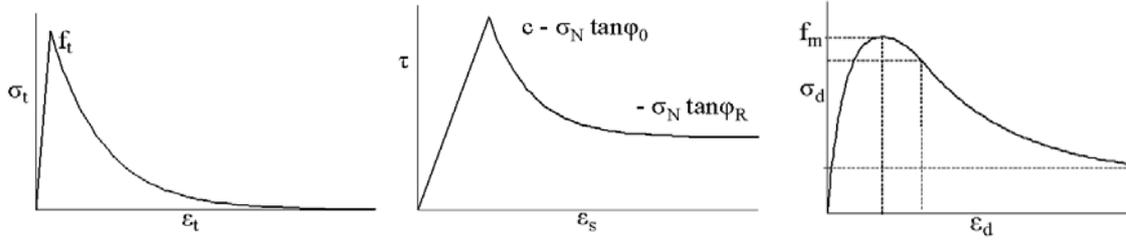
Figure 2: Stress-strain laws for the masonry material models.
